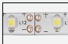
Marked cut lines every 3 LED's
